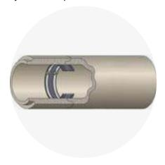
The compressive force providing the seal on either side of the joint is the result of increasing the effective diameter of the stainless steel expansion bands. The diameters of the expansion bands are increased by tightening the bolts on the WedgeLock Assemblies. This forces the corresponding wedges, which are attached to the expansion bands, away from each other increasing the expansion band diameter.
